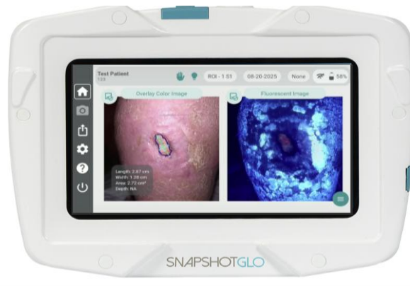
Figure 1: SnapshotGLO device displaying RGB image (L) with wound measurement alongside BAF image (R) side by side.
