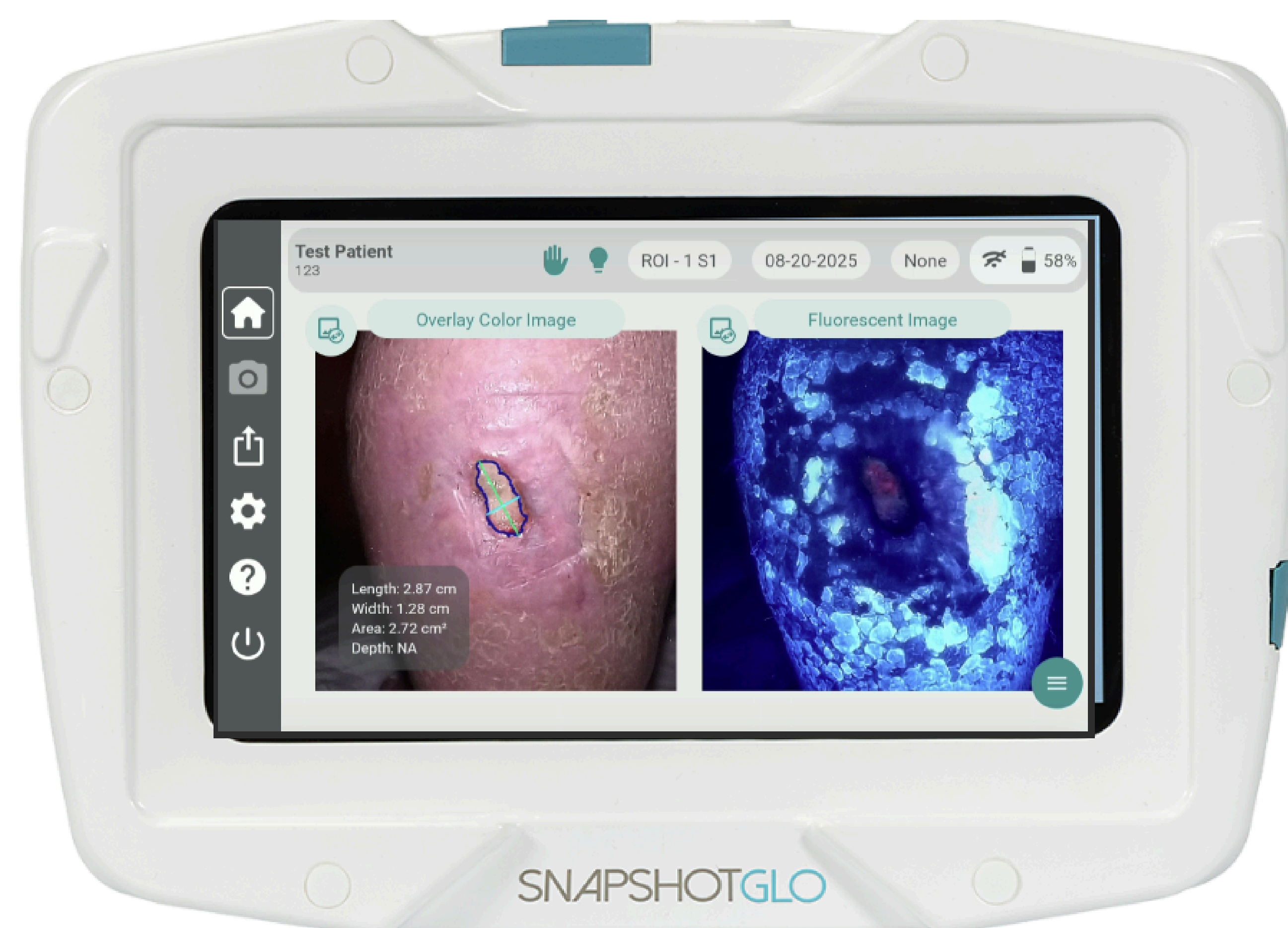
Figure: SnapshotGLO device displaying RGB image with wound measurement alongside Fluorescence image side by side.
