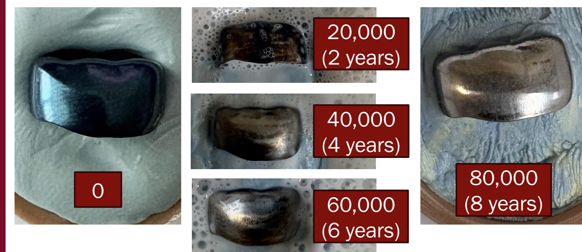
Figure 4: Blue Prismo crowns after respective number (and years equivalent) of toothbrush abrasion cycling
