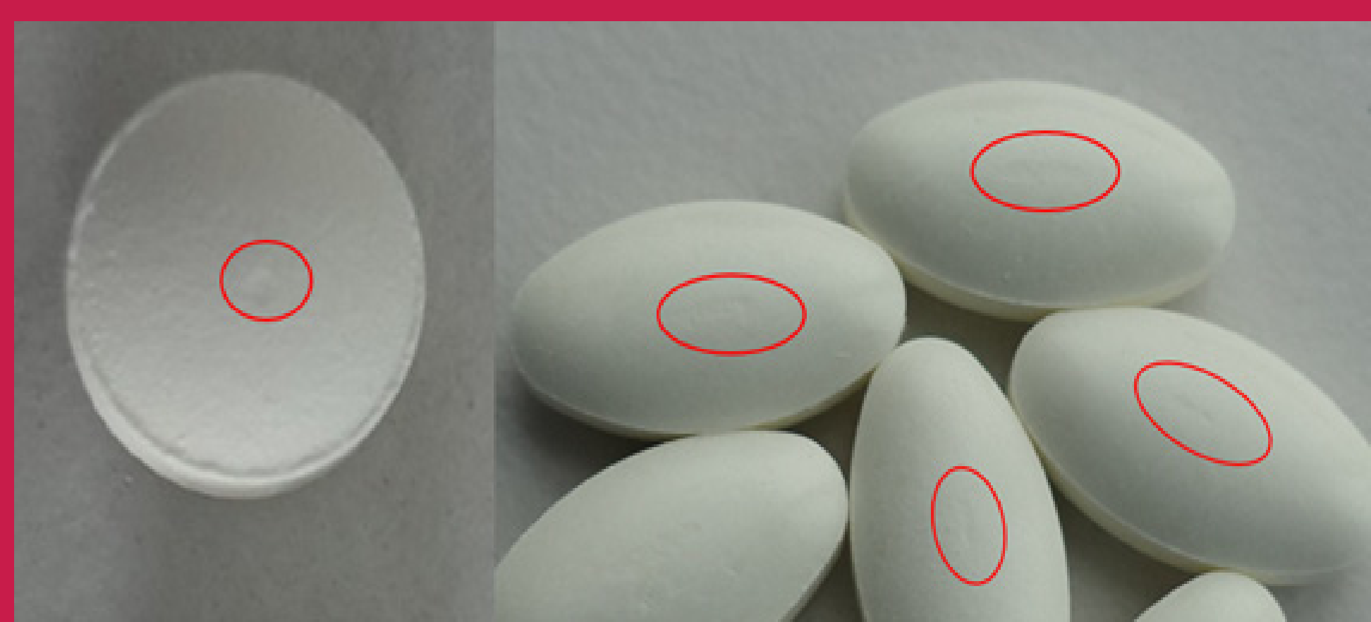
Differently sized tablets with sticking defects on their surface.
